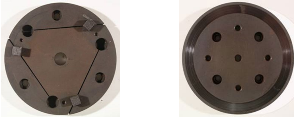
Figure I.2.2.5. Brake pad holder and tested subscale brake rotor. Source: PNNL.
