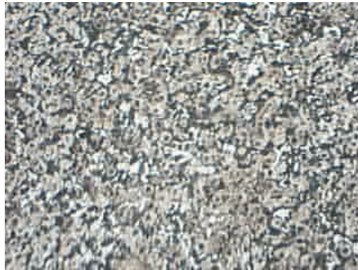
Figure II.1.6.2. Micrograph etched at 1.5 mm thickness showing typical bullseye ferrite and no carbides at 100X. Source: Skuld LLC.
