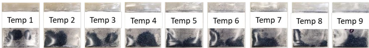
Figure II.2.7.8. Fibers bundles after carbonization. Source: ORNL.
