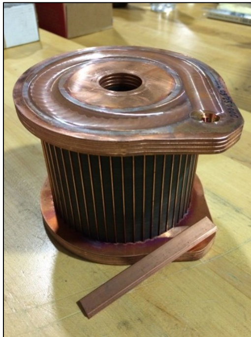
Figure I.2.1.1. Induction motor rotor and an example of a shorting bar. Source: PNNL.
