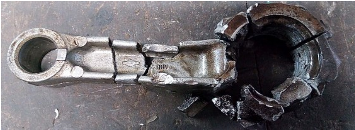
Figure I.3.5.4.1. Al connecting rod for a 4-stroke engine failed by fatigue, which subsequently impacted the crankshaft and caused catastrophic engine damage. Source: Wikipedia.
