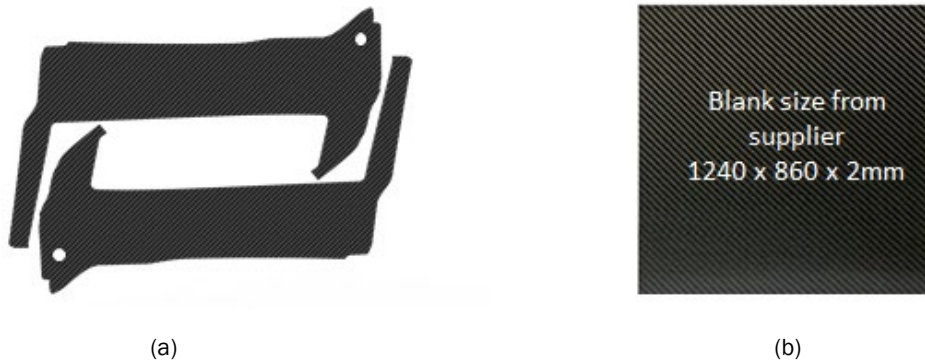
Figure II.2.4.11. (a) Inner beltline stiffener blank strategy; and (b) the blank size (1240 × 860) obtained from the supplier. Source: Clemson University.
