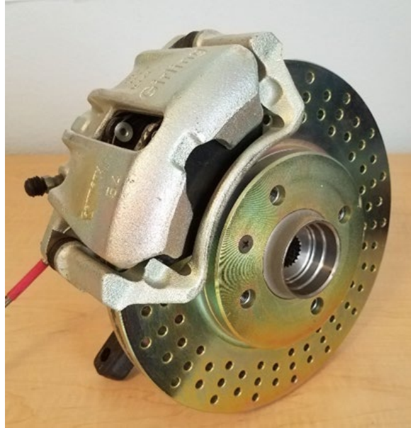
Figure I.2.2.1. Conventional brake design utilizing an Al caliper and a cast-Fe brake disc. Source: PNNL.
