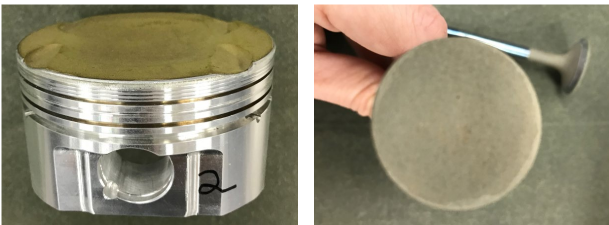
Figure I.4.1.11. Coated piston and valve hardware before testing. Source: Ford.
