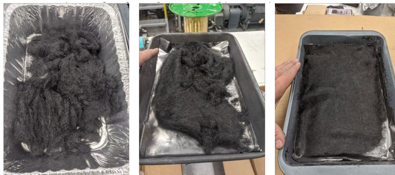
Figure II.2.7.9. Fiber mat after carbonization. Source: ORNL.
