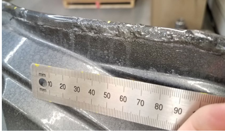
Figure II.3.5.13. Example of corrosion on CFRP-Al liftgate after 12 weeks of R-343 corrosion testing. Source: Ford.
